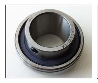
In most **KML** bearing styles the original seals and/or flingers are reinstalled after the solid lube is cured in the ball cavity. This extra sealing protection increases the service life of the bearing. It is not uncommon to double or triple the operating life of the bearing in the original application due to the superior performance of the solid lubricant coupled with the labyrinth sealing systems.
